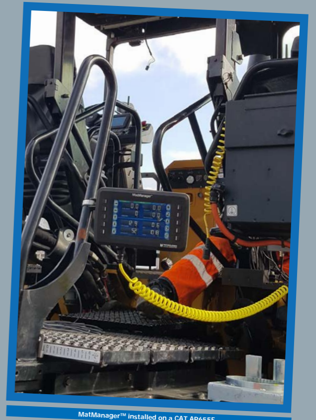
MatManager™ installed on a CAT AP655F
