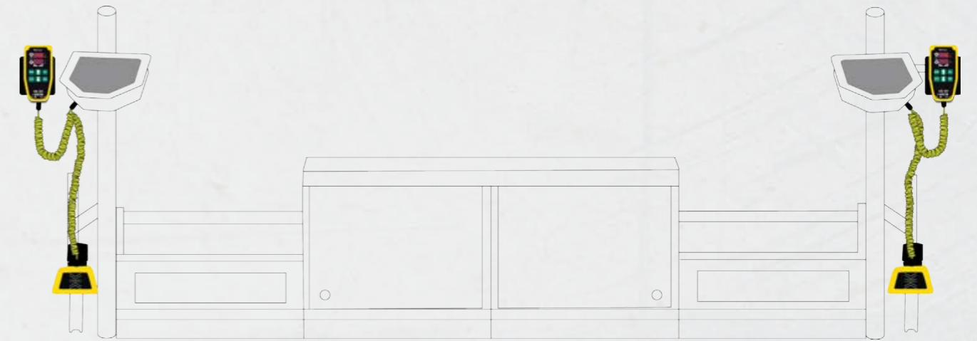
HS301 Double Grade Control Kit with G224 Multi-Sonic sensors as set up on the asphalt paver. Sensor and controller connect to the 10-pin plug of the asphalt paver with a V-Cable in each side of the screed.
